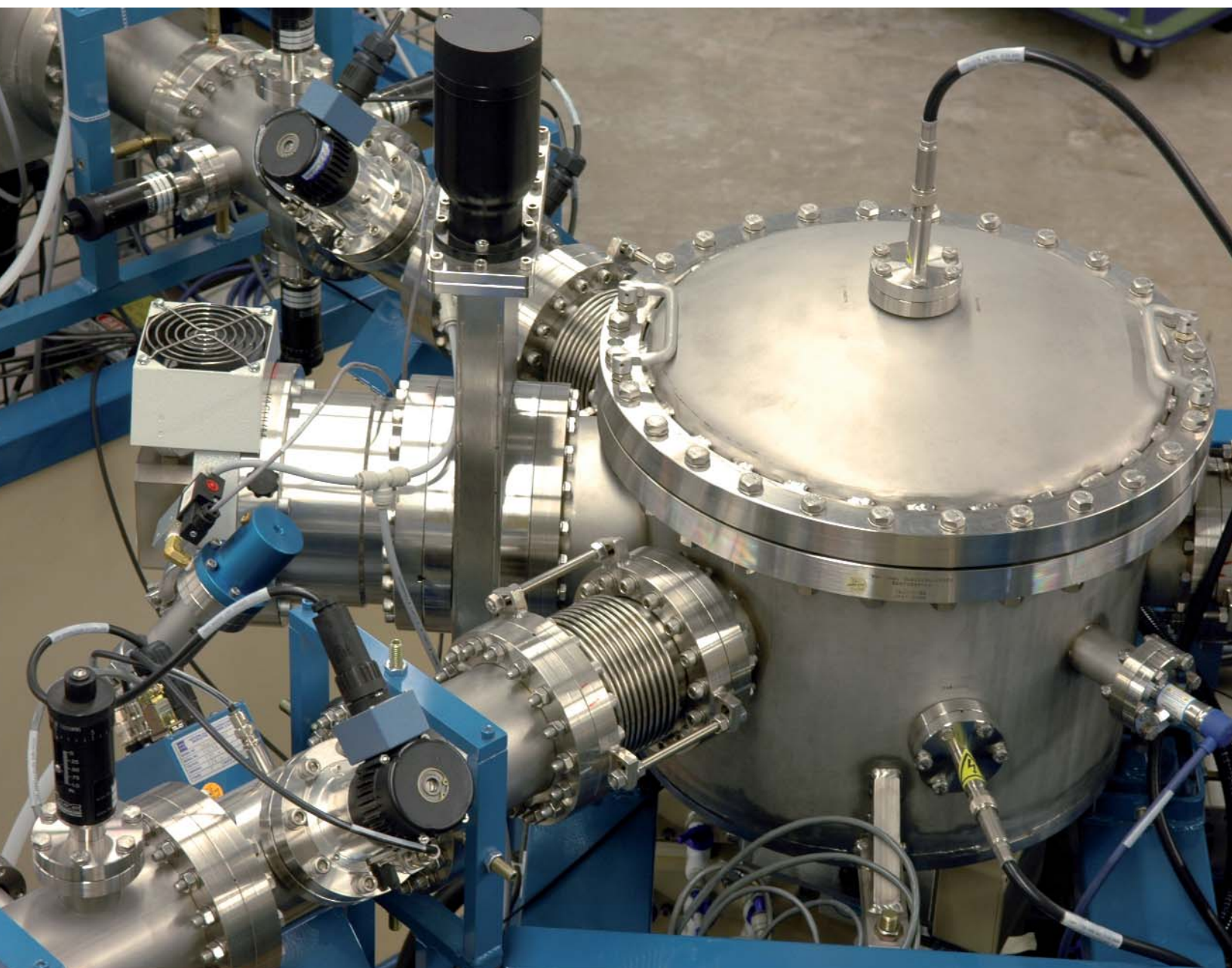
The science of dating: part of an Accelerator Mass Spectrometer used for radiocarbon dating. (Photo: Barrie Hartwell, Queens University, Belfast)
